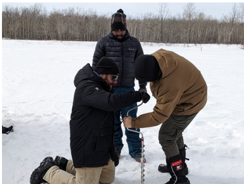
Justice Monias helps the team drill a hole in the ice so that we could measure the ice thickness
