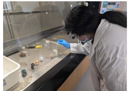
Summer Harper tests the acid resistance of various fabrics
