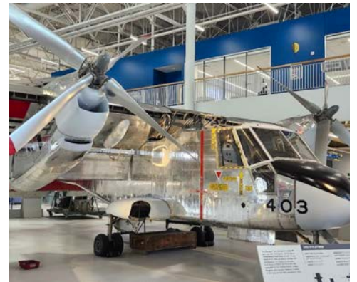
World's first tilt-wing aircraft "Canadair CL-84 Dynavert" designed in 1956
